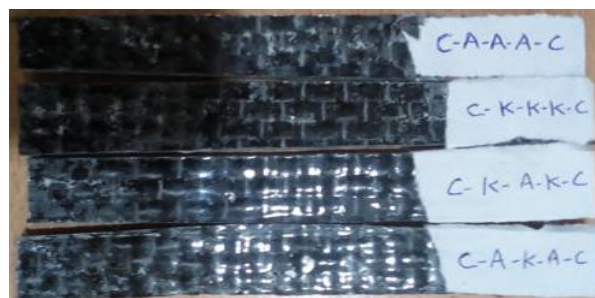
Fig.4 Flexural test specimen
