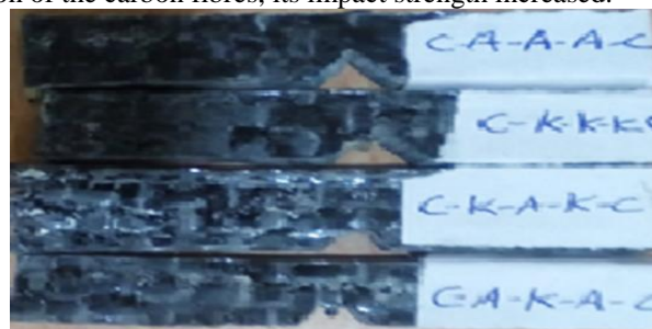
Fig.3 Impact test specimen
