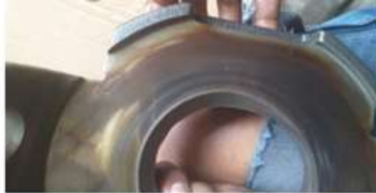
Figure 5. Abrasive wear on a wash plate surface
