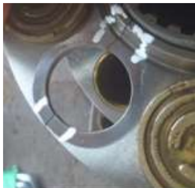
Figure 4. Cracking on slipper retainer plate
