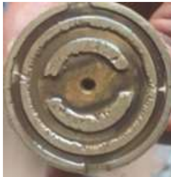
Figure 3. Abrasive wear on piston pump slipper
