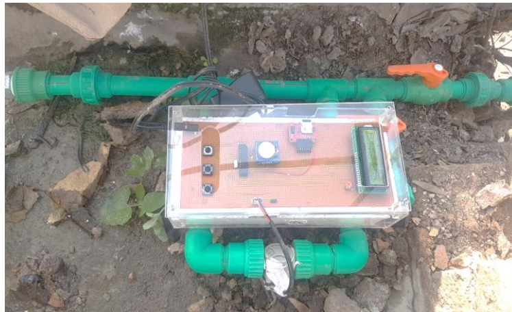
Figure.2 Arduino flow meter system
