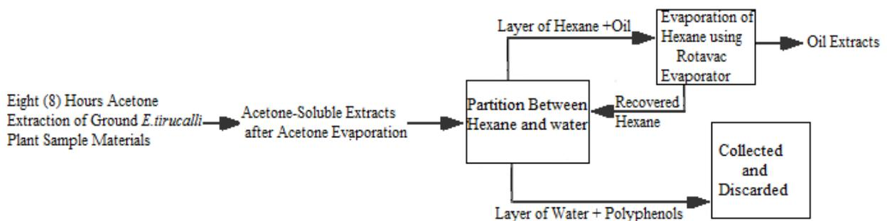
Figure 1. The extraction-Partitioning Scheme for Extraction of Oil adapted from Buchanan et al., (1978); Photi, (2005) and then Modified by the Researcher.
