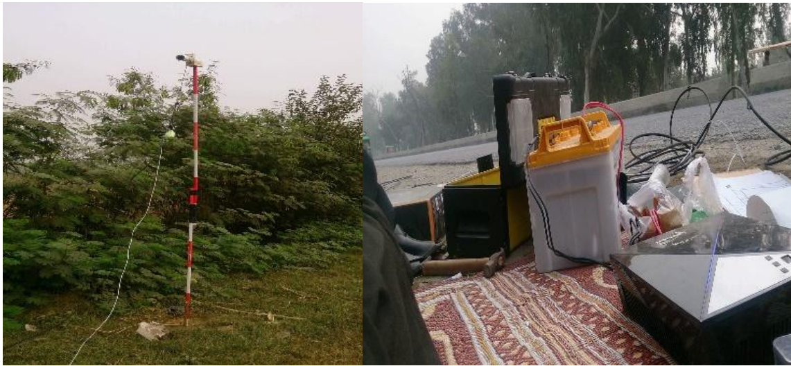
Figure 1.2 Camera and Video recording setup for average speed calculation
