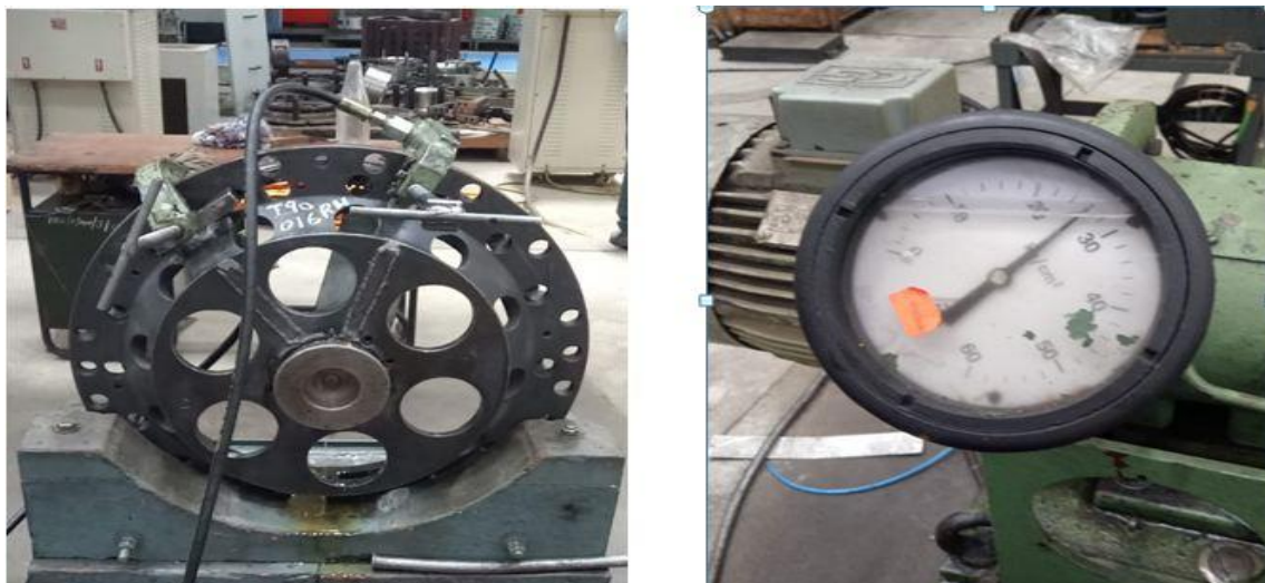
Fig. 5: Leak Test: Front Flange
