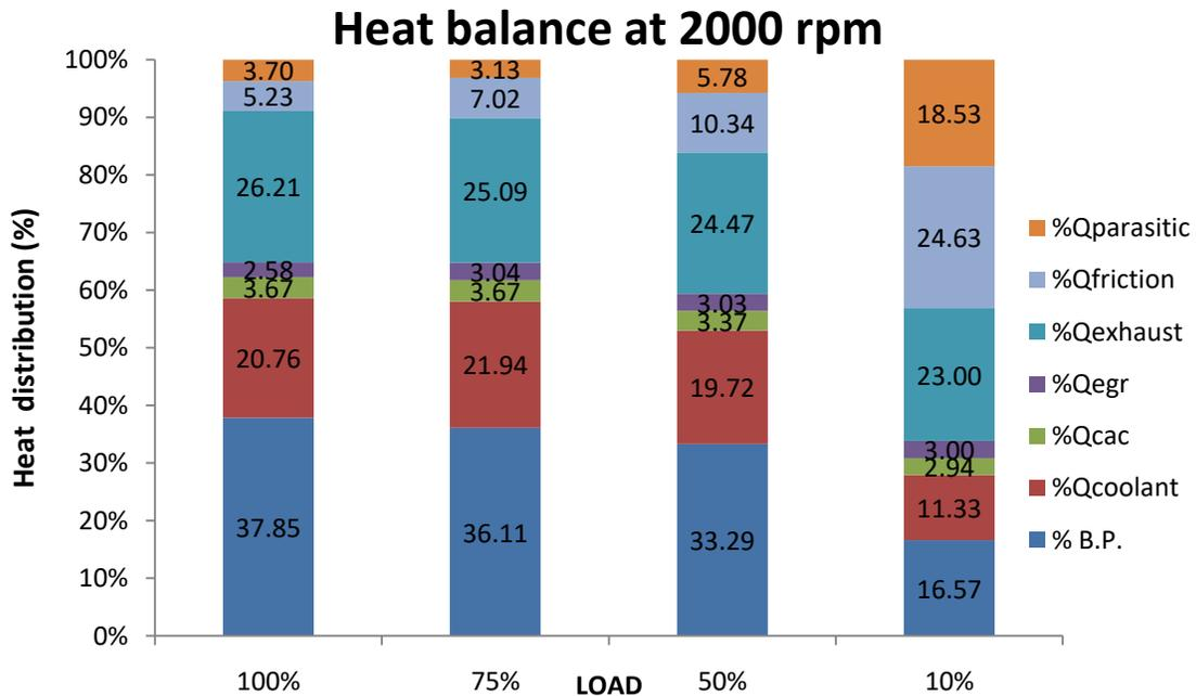
Fig. 9: Heat balance at rated speed
