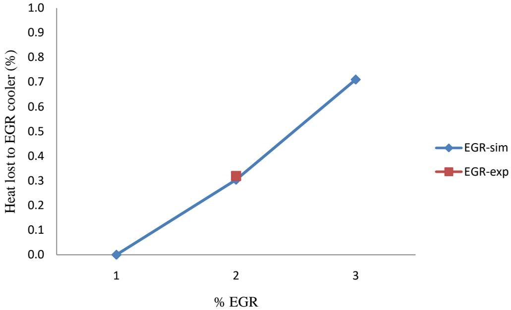
**Fig. 20: Effect of EGR on % heat lost to EGR cooler**
