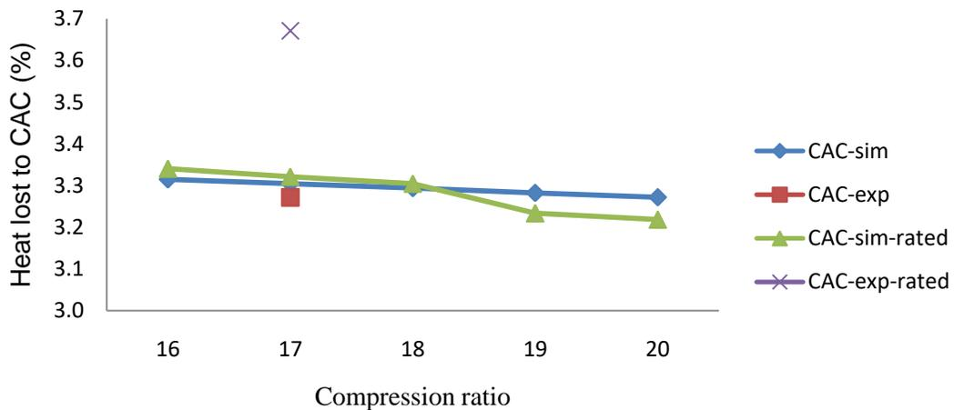
**Fig. 15: Effect of compression ratio on heat lost to CAC**
