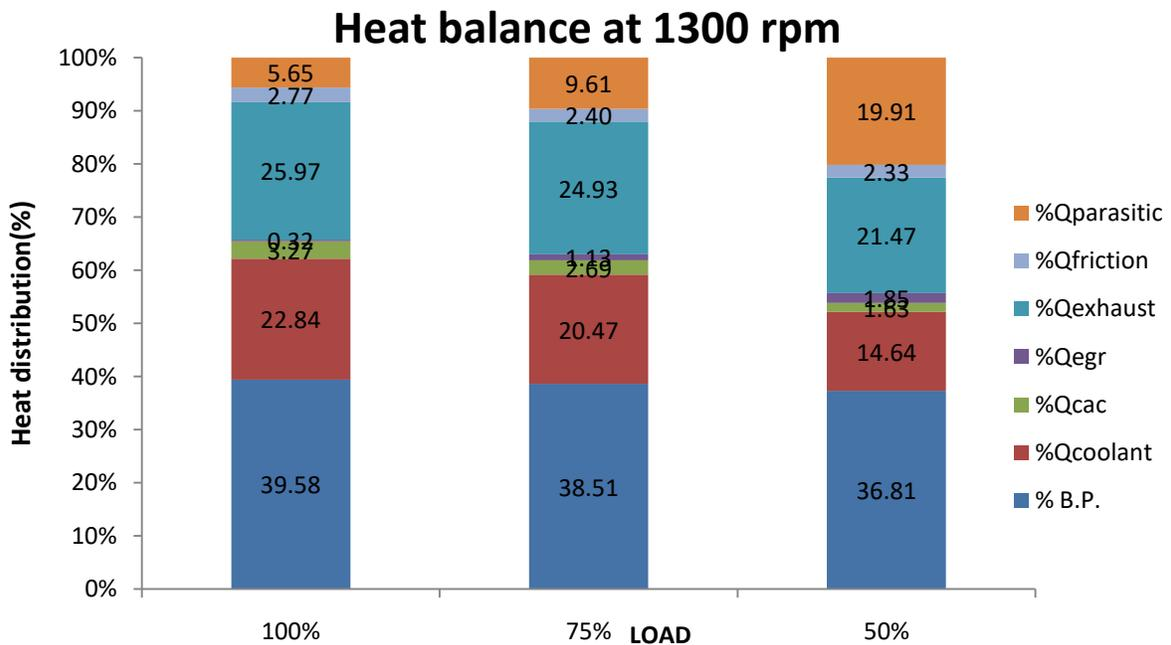
Fig. 10: Heat balance at intermediate speed
