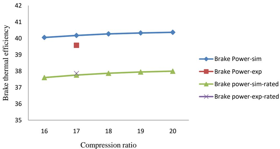
**Fig. 11: Effect of compression ratio on brake thermal efficiency**
