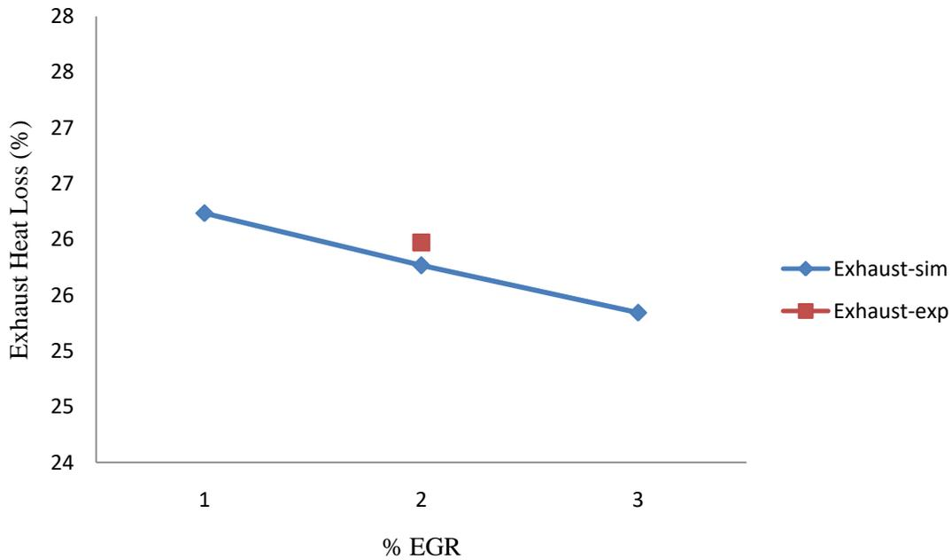
**Fig. 18: Effect of EGR on % heat lost to exhaust**
