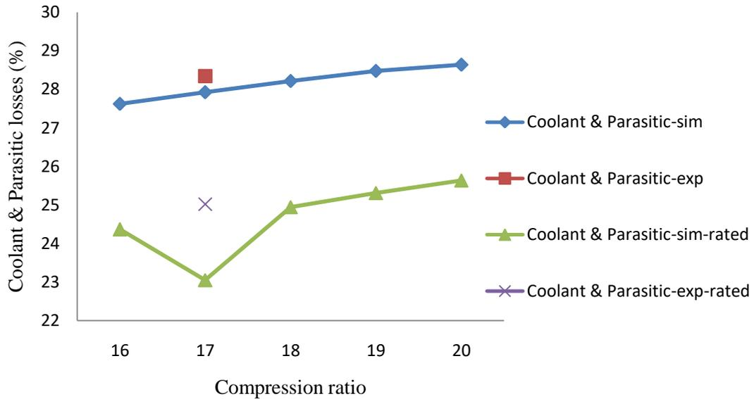
**Fig. 13: Effect of compression ratio on coolant & parasitic losses**
