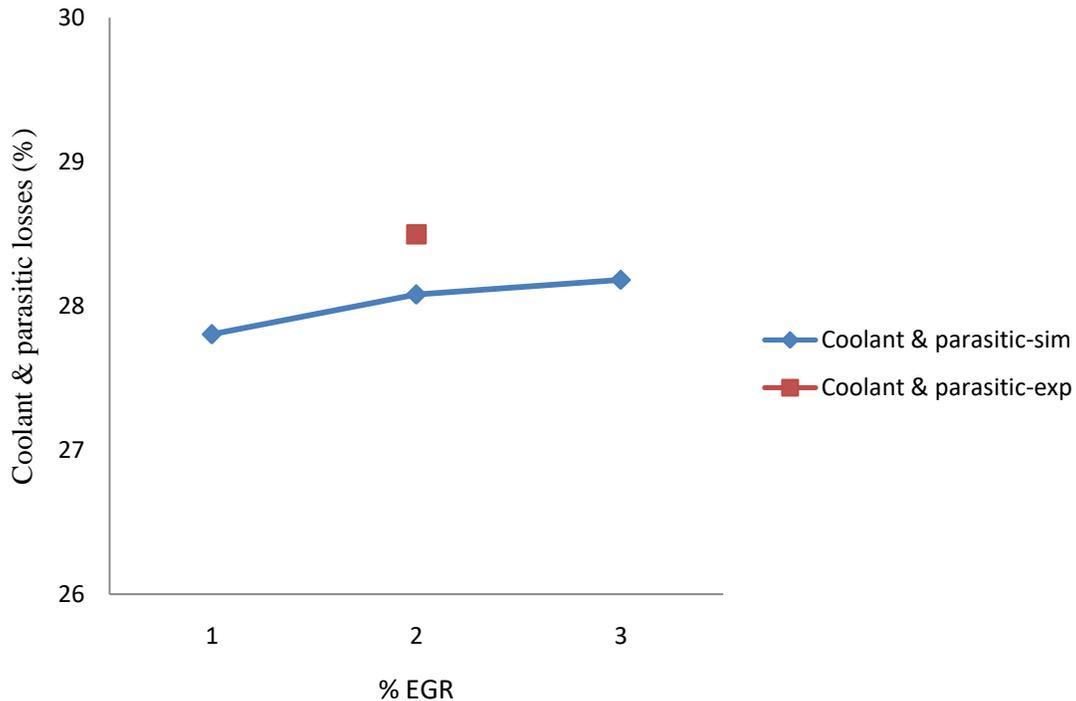
**Fig. 19: Effect of EGR on % coolant & parasitic losses**
