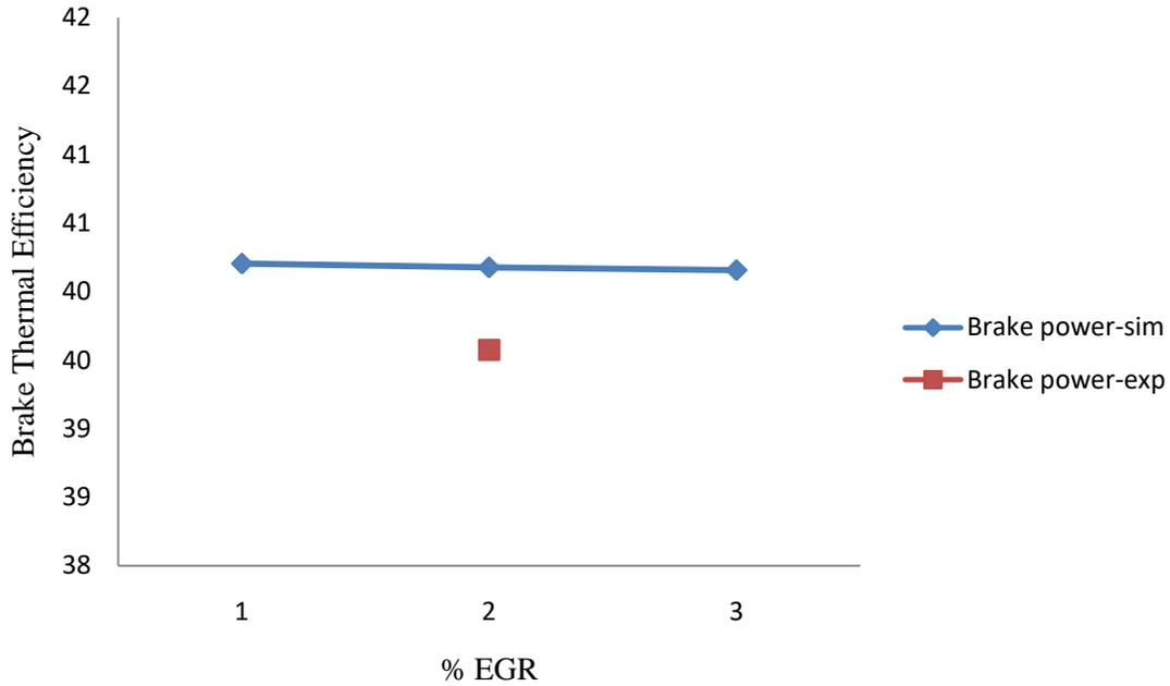
**Fig. 17: Effect of EGR on brake thermal efficiency**
