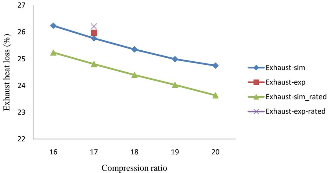
**Fig. 12: Effect of compression ratio on % exhaust heat loss**
