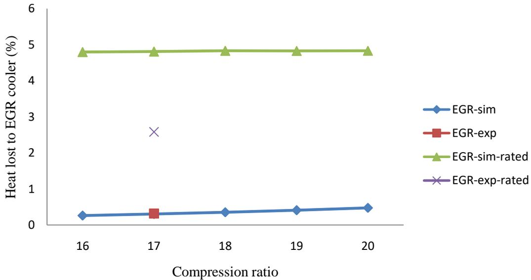
**Fig. 14: Effect of Compression Ratio on Heat Lost to EGR Cooler**
