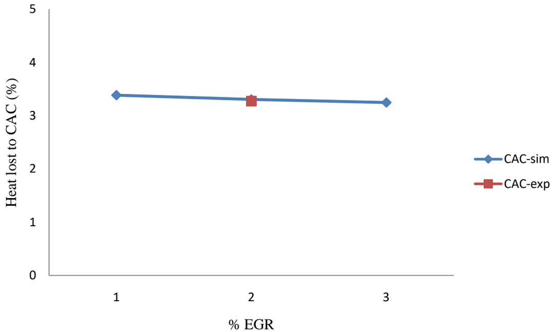
**Fig. 21: Effect of EGR rate on Heat lost to CAC**
