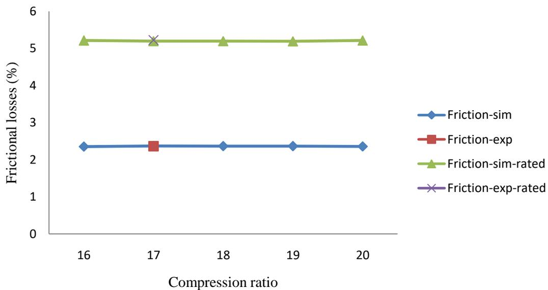
Fig. 16: Effect of compression ratio on friction losses
