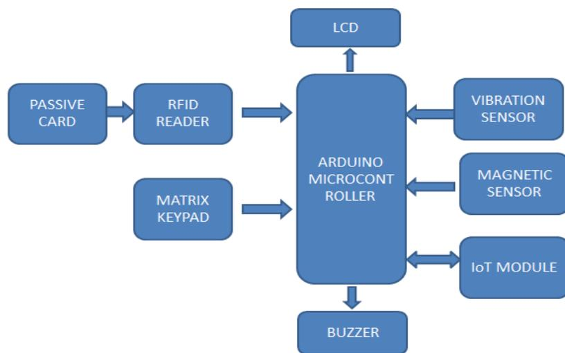
Fig.1: Block diagram of security system
